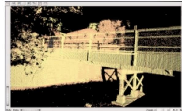
Point cloud view from scan #3. Under the foliage the historical stone embankment is clearly visible from this angle.
