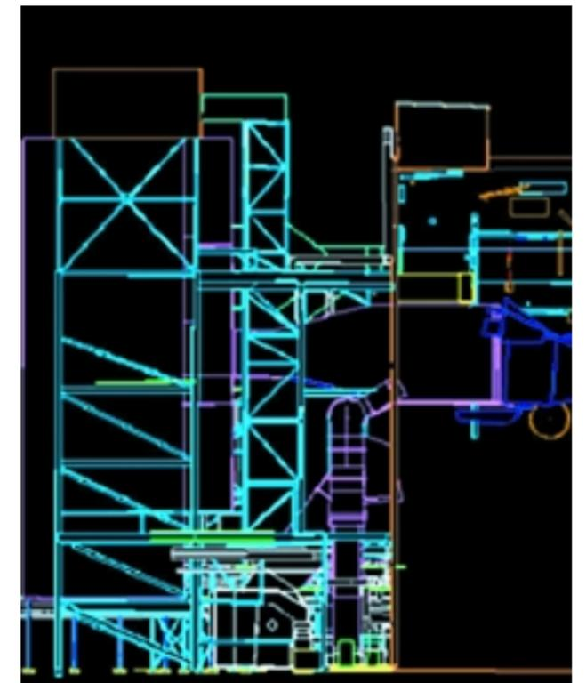
Shrinkwrap (wiremesh) view of the same structure (left) and the resulting 2D section view in Microstation (above).
