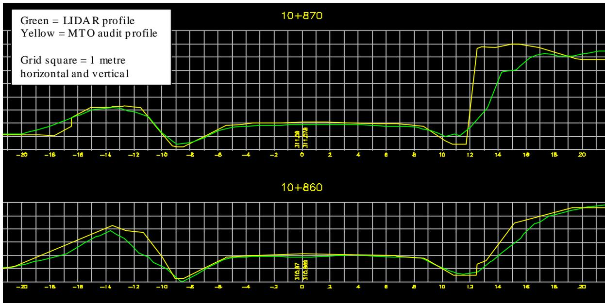
**Figure 6 - Profiles of the DTM from LIDAR (green) and MTO audits (yellow)**
