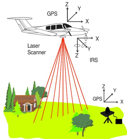
**Figure 2 - LIDAR Positioning System**
