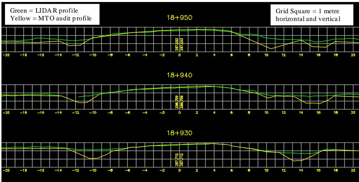
**Figure 4 - Profiles of the DTM from LIDAR (green) and MTO audits (yellow)**
