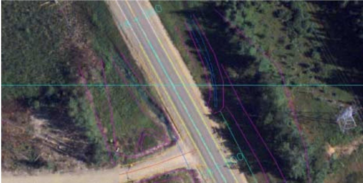
**Figure 3 - Digital Imagery overlaid with MTO audit strings in Ditch Area**
