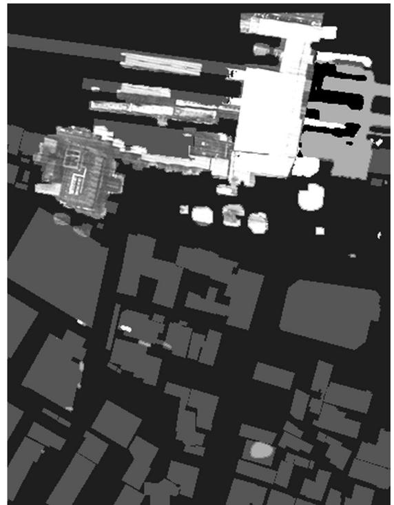
Fig. 6. An orthoimage of the study area overlaid with the change image of Fig. 4 and existing building database. Grey areas are building data in the building database. Only parts of the orthoimage where changes were identified during the change detection process are displayed to facilitate the database revision and inspection process by the operator.
