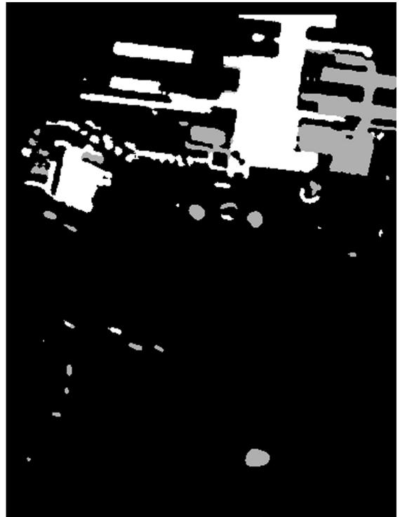
Fig. 4. Changes detected in Fig. 3. The Fig. 3 image was transformed into a binary image with a threshold value of 1 m and then the noise was removed by using a simple noise reduction filter.
