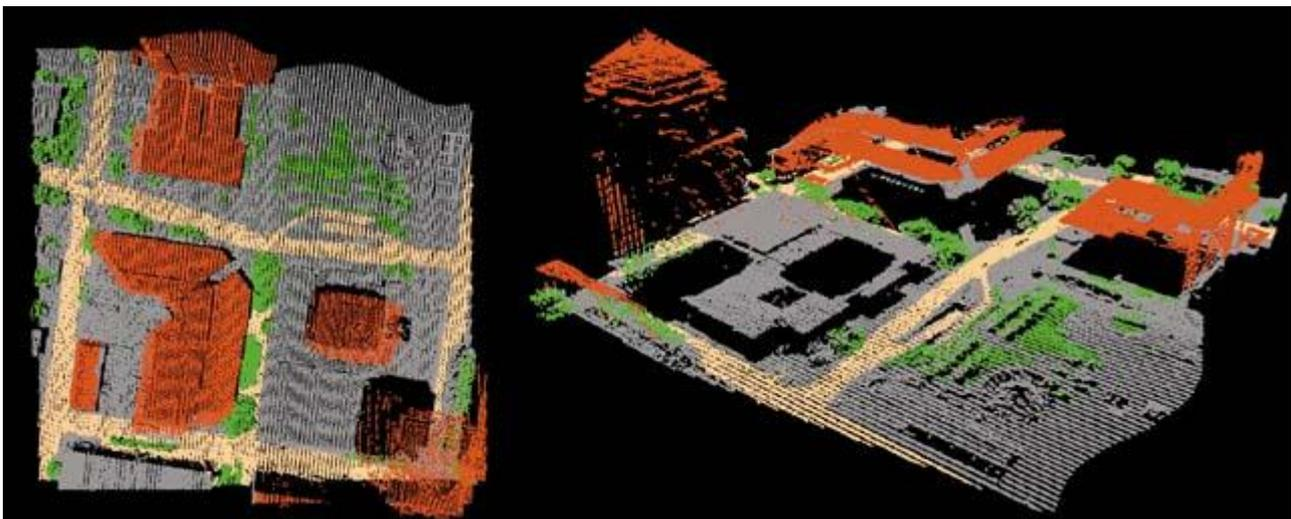
Figure 1. Lidar returns classified by features, roads, surface, buildings and vegetation, using SILC technology
