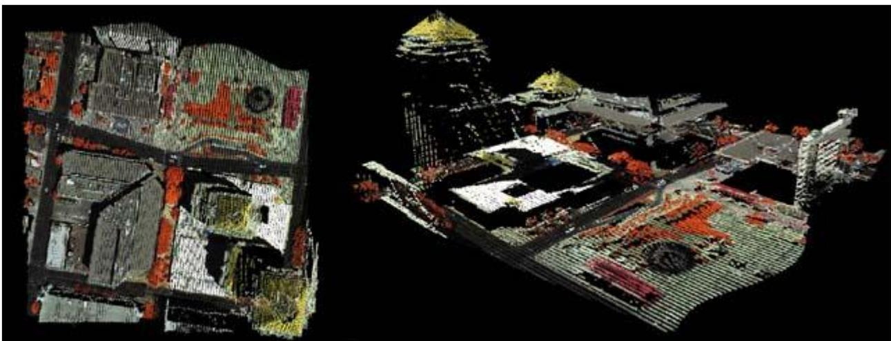
Figure 3. Unfiltered Lidar data colored with SILC (CIR values), plan view and oblique.
