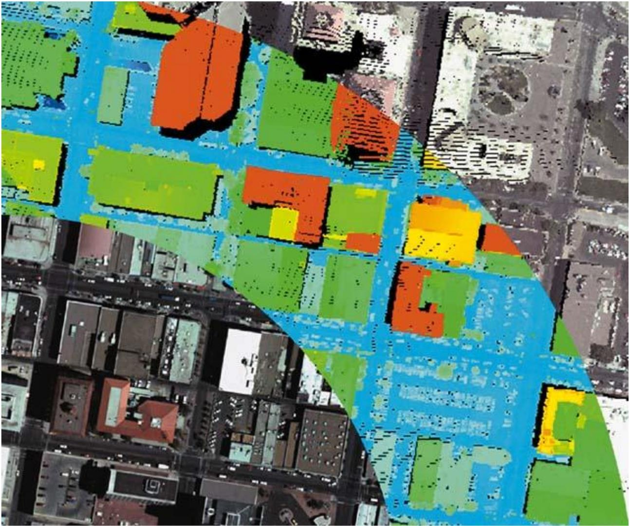
**Figure 2. Inner circle – color digital imagery. Middle circle – Lidar data colored by elevation. Outer circle – SILC laser points attributed with SILC RGB values.**
